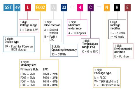
Temperature ranges: 0 to 85°C on SST products (0 to 70°C on ST's, some extended -20 to 85°C)
