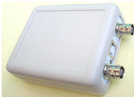
Connect one end of USB cable to the USB connection of oscillograph, and the other end to computer. The light will on if the connection is right.
