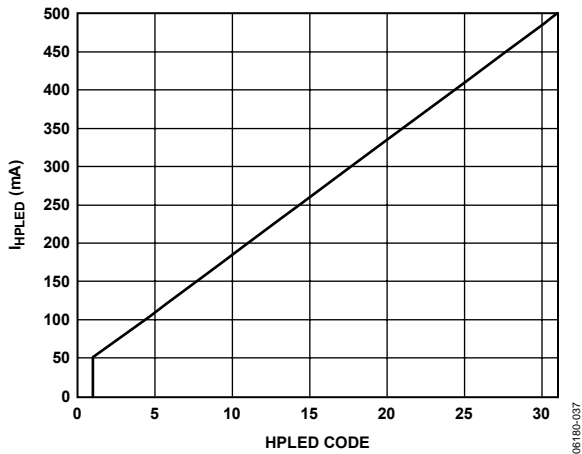
Figure 11. HPLED Current vs. HPLED Code, I^2C Mode, SETF = V_{DD}
