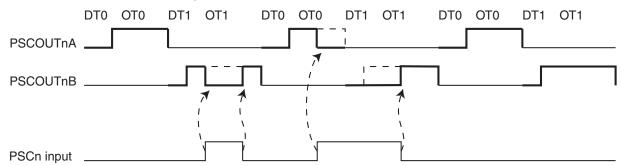
Figure 17-13. PSC behaviour versus PSCn Input A or Input B in fault mode 4.
