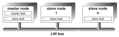
The master task decides when and which frame shall be transferred on the bus. The slave tasks provide the data transported by each frame. Both the master task and the slave task are parts of the Frame handler.
