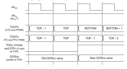
Figure 15-13 on page 117 shows the same timing data, but with the prescaler enabled.
