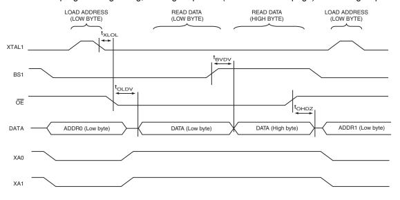
Note: 1. The timing requirements shown in Figure 27-7 on page 287 (that is, t<sub>DVXH</sub>, t<sub>XHXL</sub>, and t<sub>XLDX</sub>) also apply to reading operation.
