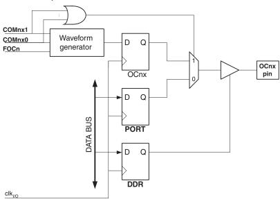
The general I/O port function is overridden by the Output Compare (OC0x) from the Waveform Generator if either of the COM0x1:0 bits are set. However, the OC0x pin direction (input or output) is still controlled by the Data Direction Register (DDR) for the port pin. The Data Direction Register bit for the OC0x pin (DDR\_OC0x) must be set as output before the OC0x value is visible on the pin. The port override function is independent of the Waveform Generating mode.
