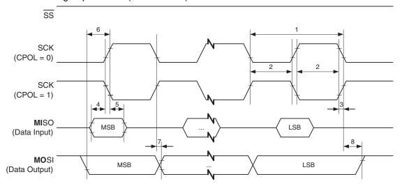
Figure 28-4. SPI interface timing requirements (Slave mode).
