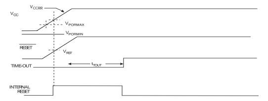
Figure 10-3. MCU start-up, RESET extended externally.
