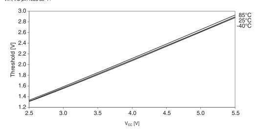
Figure 29-8. I/O pin input threshold voltage versus  $V_{CC}$ . VIL, I/O pin read as '0'.
