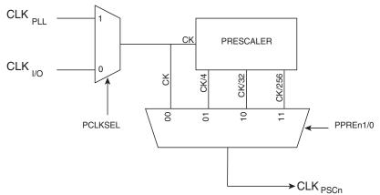
PCLKSELn bit in PSC Control Register (PCTL) is used to select the clock source.
