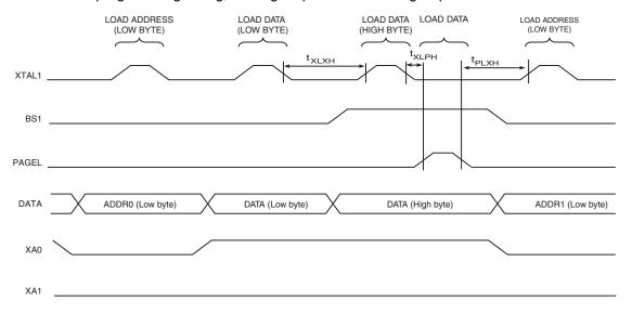
Note: 1. The timing requirements shown in Figure 27-7 (that is, t<sub>DVXH</sub>, t<sub>XHXL</sub>, and t<sub>XLDX</sub>) also apply to loading operation.
