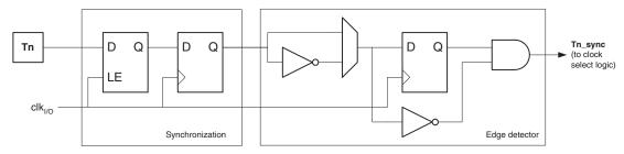
The synchronization and edge detector logic introduces a delay of 2.5 to 3.5 system clock cycles from an edge has been applied to the Tn/T0 pin to the counter is updated.
