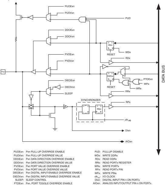
Note: 1. WRx, WPx, WDx, RRx, RPx, and RDx are common to all pins within the same port. clk<sub>I/O</sub>, SLEEP, and PUD are common to all ports. All other signals are unique for each pin.
