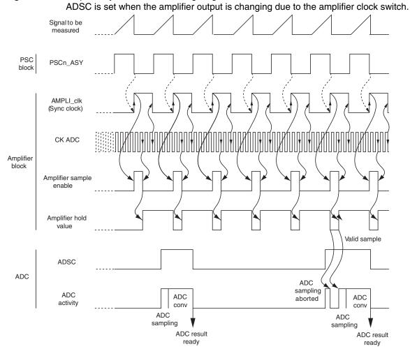
Figure 21-16. Amplifier synchronization timing diagram.
