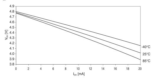
Figure 29-6. I/O pin output voltage versus source current.
