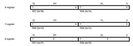
In the different addressing modes these address registers have functions as fixed displacement, automatic increment, and automatic decrement (see the "Instruction set summary" on page 319 for details).
