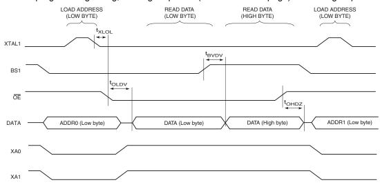
Note: 1. The timing requirements shown in Figure 28-5 on page 301 (that is,  $t_{DVXH}$ ,  $t_{XHXL}$ , and  $t_{XLDX}$ ) also apply to reading operation.
