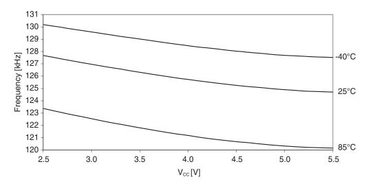
Figure 29-18. Watchdog oscillator frequency versus temperature.
