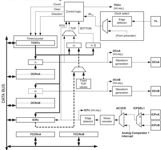
Figure 15-1. 16-bit Timer/Counter block diagram (1).
