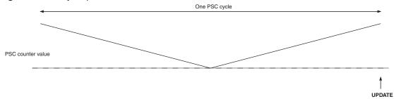
Figure 17-2 on page 129 and Figure 17-3 graphically illustrate the values held in the PSC counter. Centered mode is like One Ramp mode which counts down and then up.
