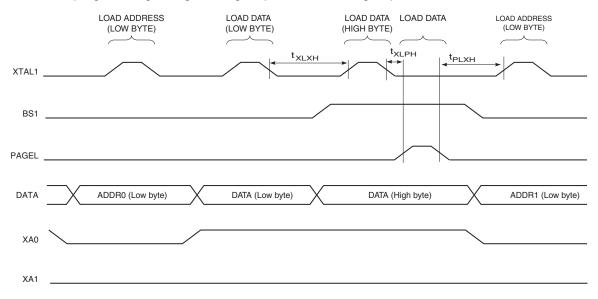
Note: 1. The timing requirements shown in Figure 28-5 (that is,  $t_{DVXH}$ ,  $t_{XHXL}$ , and  $t_{XLDX}$ ) also apply to loading operation.
