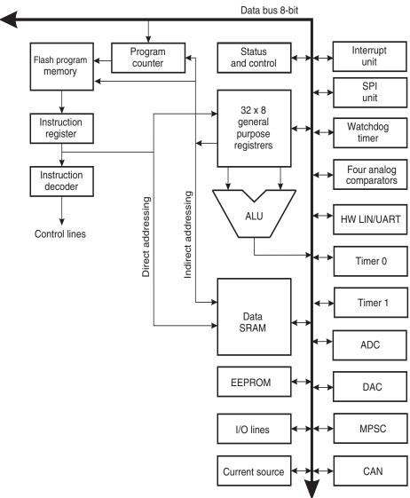
The AVR core combines a rich instruction set with 32 general purpose working registers. All the 32 registers are directly connected to the Arithmetic Logic Unit (ALU), allowing two independent registers to be accessed in one single instruction executed in one clock cycle. The resulting architecture is more code efficient while achieving throughputs up to ten times faster than conventional CISC microcontrollers.
