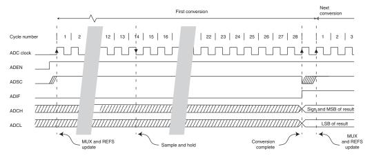
Figure 21-5. ADC timing diagram, single conversion.
