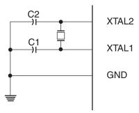
The oscillator can operate in three different modes, each optimized for a specific frequency range. The operating mode is selected by the fuses CKSEL3..1 as shown in Table 8-3 on page 28.
