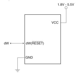
Figure 25-1 shows the schematic of a target MCU, with debugWIRE enabled, and the emulator connector. The system clock is not affected by debugWIRE and will always be the clock source selected by the CKSEL Fuses.
