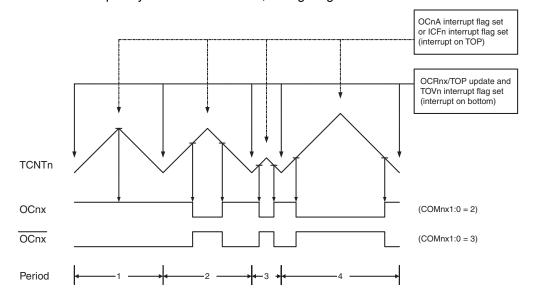
The Timer/Counter Overflow Flag (TOVn) is set at the same timer clock cycle as the OCRnx Registers are updated with the double buffer value (at BOTTOM). When either OCRnA or ICRn is used for defining the TOP value, the OCnA or ICFn Flag is set when TCNTn has reached TOP. The Interrupt Flags can then be used to generate an interrupt each time the counter reaches the TOP or BOTTOM value.
