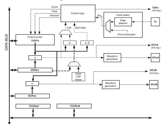
Figure 14-1. 8-bit timer/counter block diagram.
