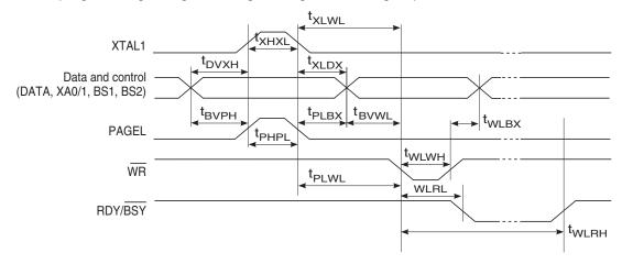
**Figure 28-6.** Parallel programming timing, loading sequence with timing requirements <sup>(1)</sup>.
