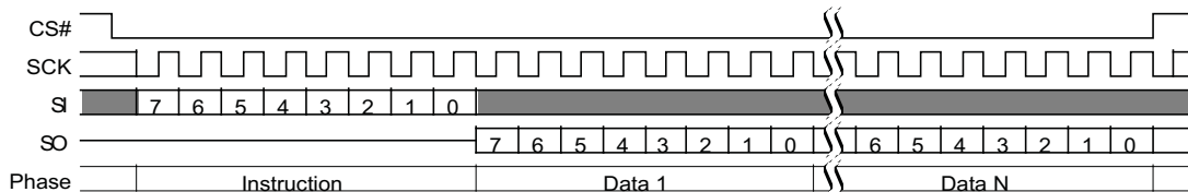
Figure 9.70 Password Read (PASSRD E7h) Command Sequence
