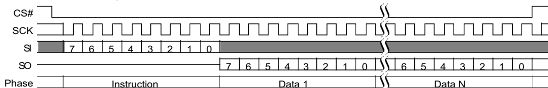
Figure 9.2 Read Identification (RDID 9Fh) Command Sequence
