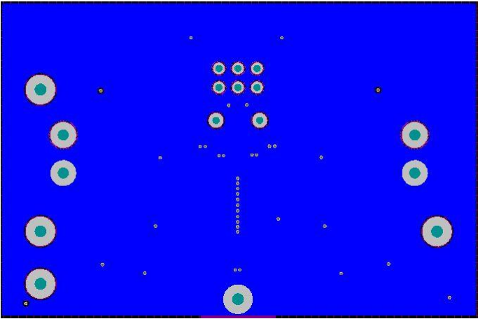
Figure 2. PCB Copper Layout & Silk Screen – Bottom
