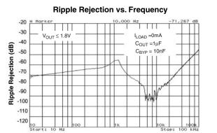
**Ripple Rejection vs. Frequency**
