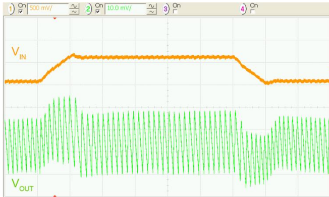
Figure 20. Line Transient 3.3 V_{IN} to 3.9 V_{IN} , 50 mA Load, 10 \mu\text{s}/\text{div} .
