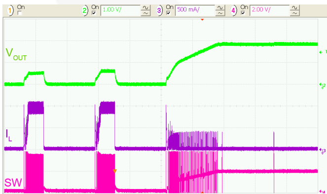
Figure 37. Overload Recovery to Light Load, 50\ \mu\text{s}/\text{div} .
