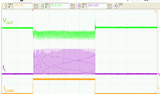
Figure 30. Load Transient 0 to 150 mA, 4.5 V_{IN}
