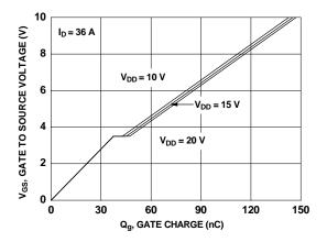
Figure 7. Gate Charge Characteristics
