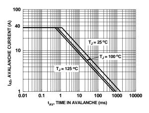
Figure 9. Unclamped Inductive Switching Capability
