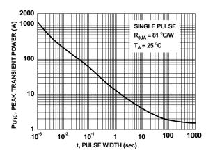
Figure 12. Single Pulse Maximum Power Dissipation
