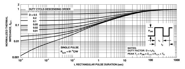
Figure 13. Junction-to-Ambient Transient Thermal Response Curve
