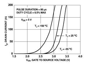
Figure 5. Transfer Characteristics
