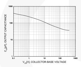
Figure 3. Collector Output Capacitance
