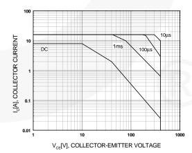
Figure 6. Forward Biased Safe Operating Area
