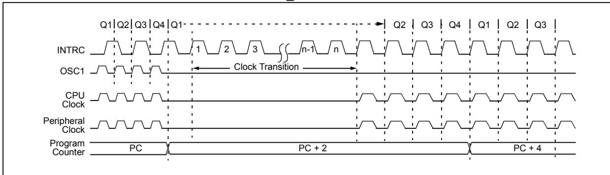
**FIGURE 4-4: TRANSITION TIMING FROM RC\_RUN MODE TO PRI\_RUN MODE**
