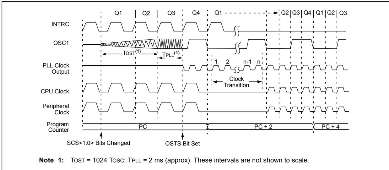
**Note 1:**  $T_{OST} = 1024 T_{OSC}$ ;  $T_{PLL} = 2 \text{ ms}$  (approx). These intervals are not shown to scale.
