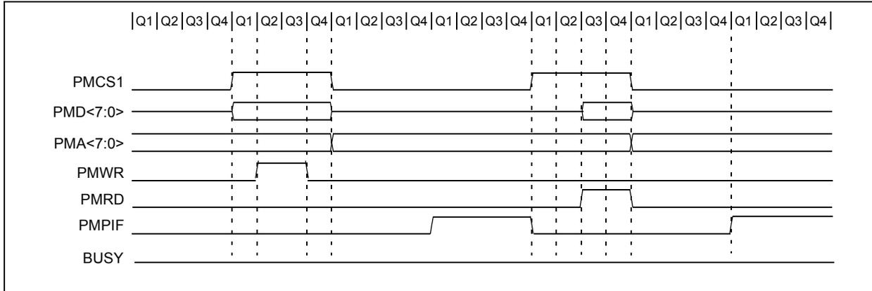
**FIGURE 11-13: READ TIMING, 8-BIT DATA, PARTIALLY MULTIPLEXED ADDRESS**
