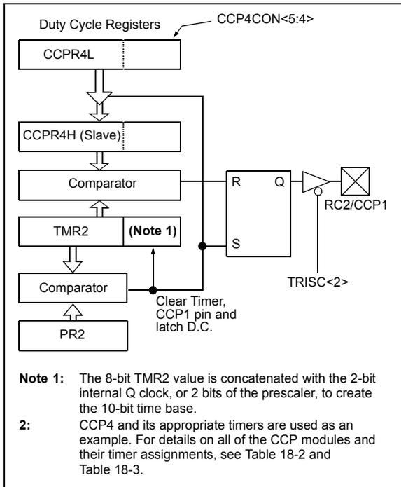
A PWM output (Figure 18-4) has a time base (period) and a time that the output stays high (duty cycle). The frequency of the PWM is the inverse of the period (1/period).
