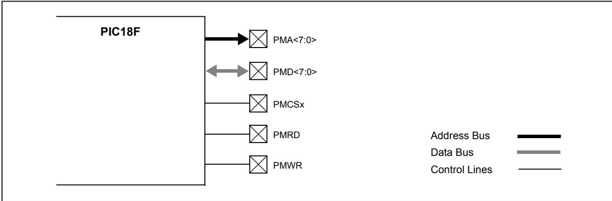
**FIGURE 11-10: PARTIALLY MULTIPLEXED ADDRESSING MODE
