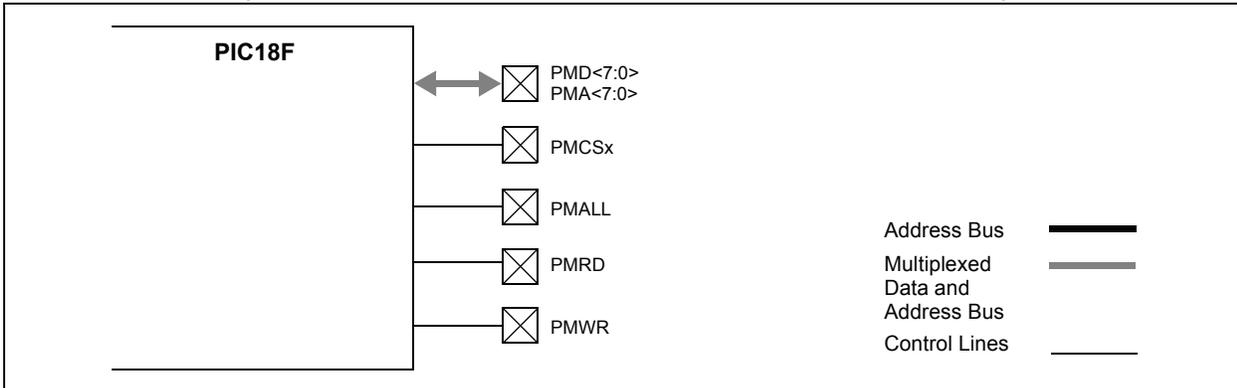
**FIGURE 11-11: FULLY MULTIPLEXED ADDRESSING MODE
