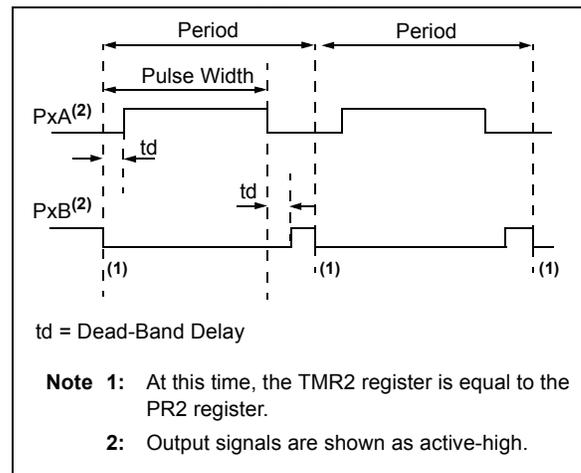
**FIGURE 19-15: EXAMPLE OF HALF-BRIDGE APPLICATIONS**
