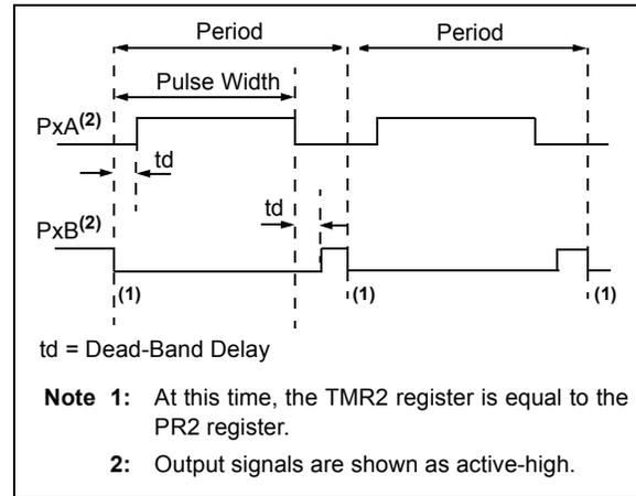
**FIGURE 19-7: EXAMPLE OF HALF-BRIDGE APPLICATIONS**
