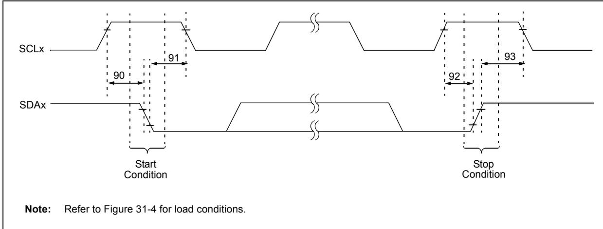
**TABLE 31-26: MSSPx I<sup>2</sup>C™ BUS START/STOP BITS REQUIREMENTS**
