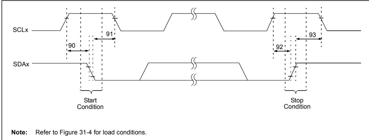
**TABLE 31-24: I<sup>2</sup>C™ BUS START/STOP BITS REQUIREMENTS (SLAVE MODE)**
