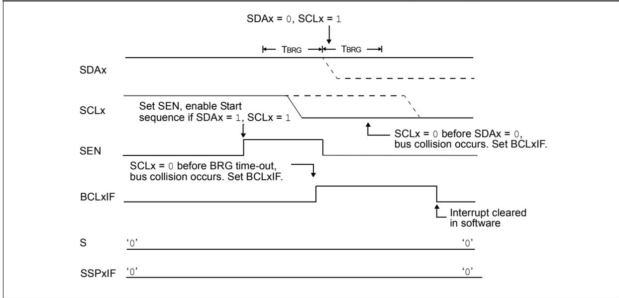
**FIGURE 20-30: BRG RESET DUE TO SDAx ARBITRATION DURING START CONDITION**
