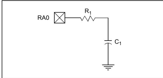
A timer can be used to measure the charge time and discharge time of the capacitor. The charge time can then be adjusted to provide the desired interrupt delay. This technique will compensate for the affects of temperature, voltage and component accuracy. The ULPWU peripheral can also be configured as a simple Programmable Low-Voltage Detect (LVD) or temperature sensor.
