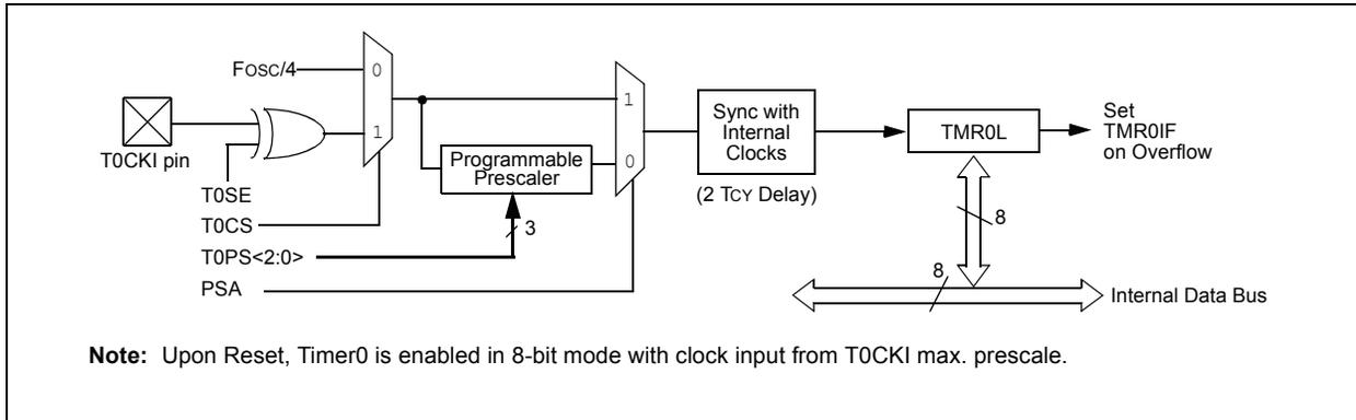
**FIGURE 12-2: TIMER0 BLOCK DIAGRAM (16-BIT MODE)**
