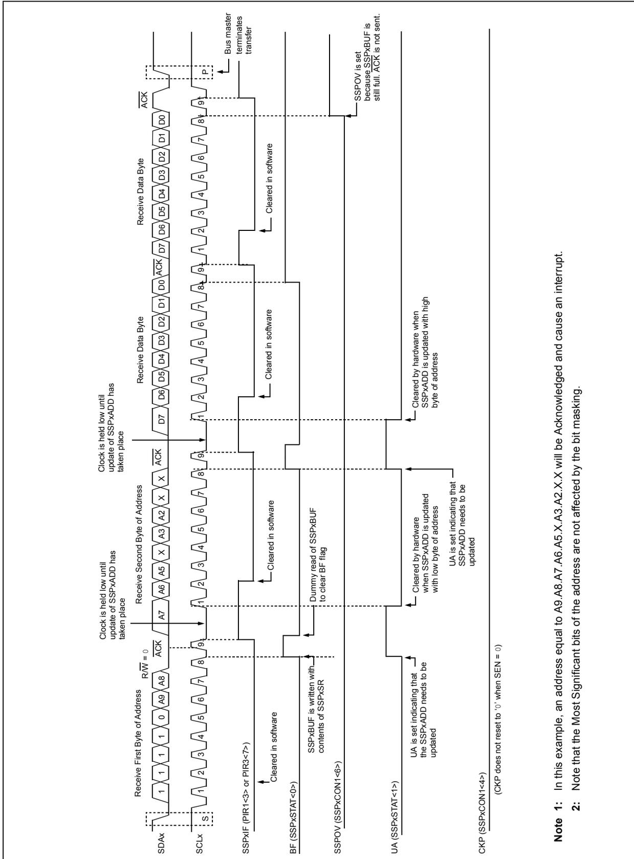
FIGURE 20-12: I<sup>2</sup>C™ SLAVE MODE TIMING WITH SEN = 0 (RECEPTION, 10-BIT ADDRESS)
