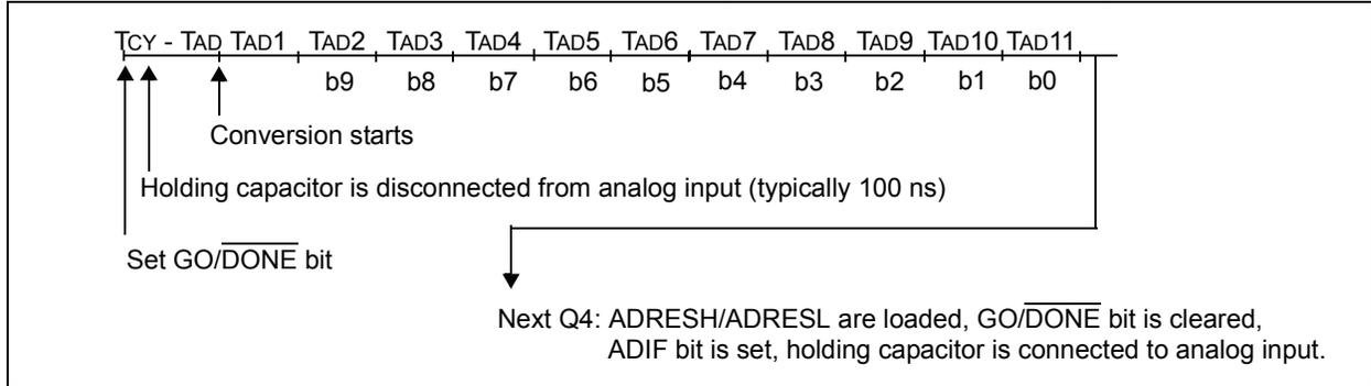
**FIGURE 22-4: A/D CONVERSION TAD CYCLES (ACQT<2:0> = 010, TACQ = 4 TAD)**
