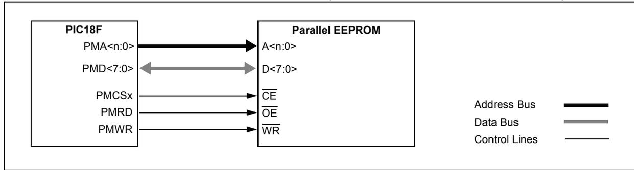
**FIGURE 11-31: PARALLEL EEPROM EXAMPLE (UP TO 15-BIT ADDRESS, 16-BIT DATA)**
