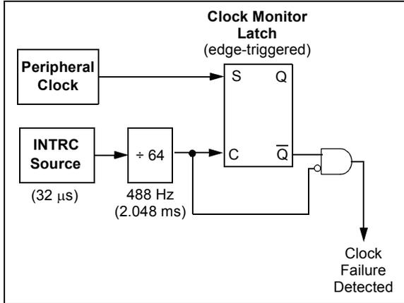
Clock failure is tested for on the falling edge of the sample clock. If a sample clock falling edge occurs while the clock monitor is still set, and a clock failure has been detected (Figure 28-5), the following results:
