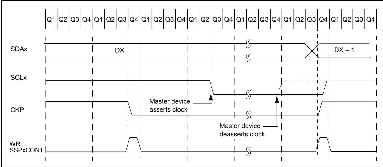
**FIGURE 20-15: I<sup>2</sup>C™ SLAVE MODE TIMING WITH SEN = 1 (RECEPTION, 7-BIT ADDRESS)**
