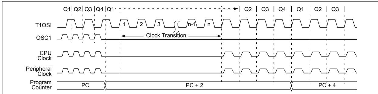
**FIGURE 4-2: TRANSITION TIMING FROM SEC\_RUN MODE TO PRI\_RUN MODE (HSPLL)**
