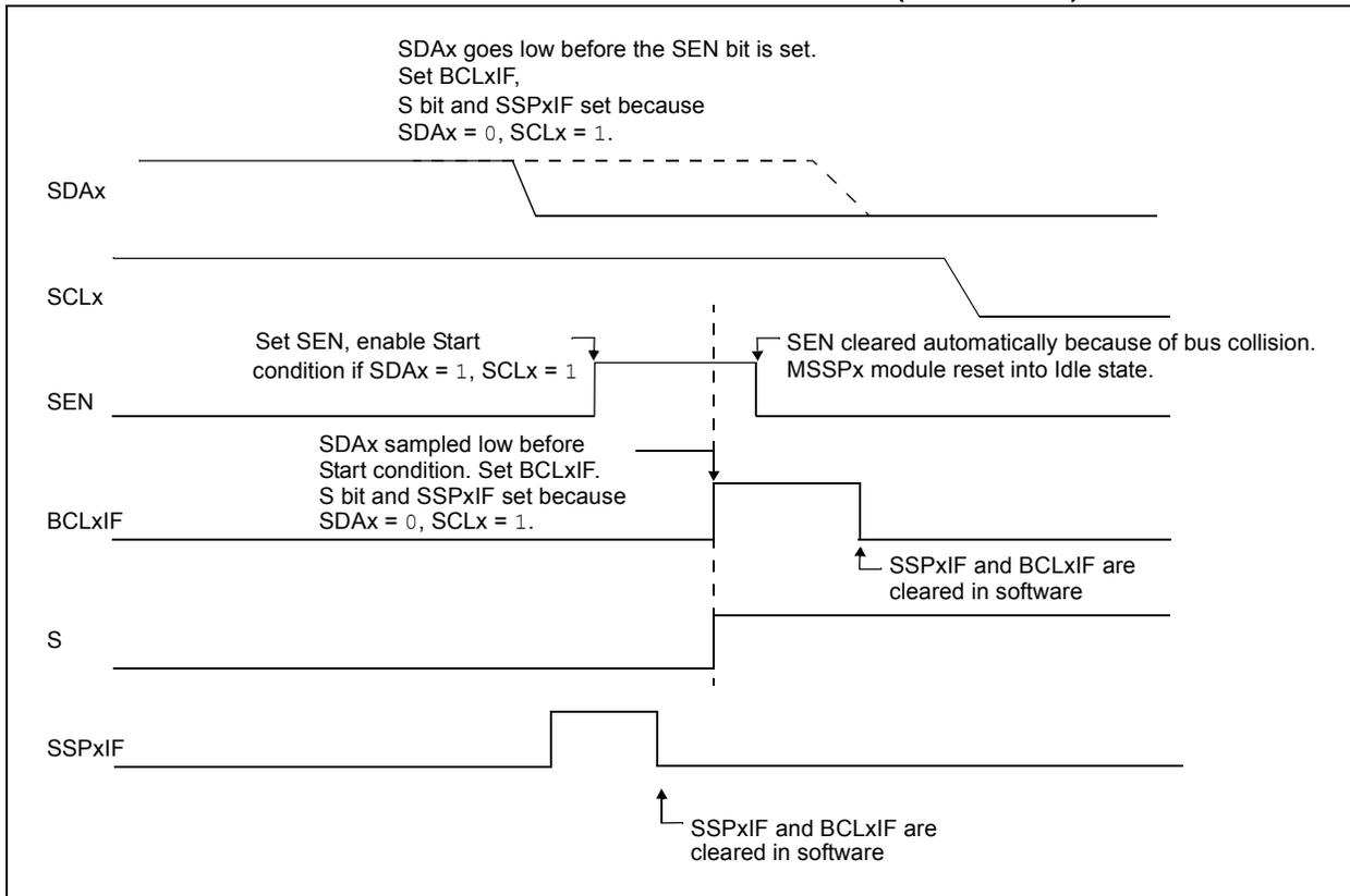
**FIGURE 20-29: BUS COLLISION DURING START CONDITION (SCLx = 0)**
