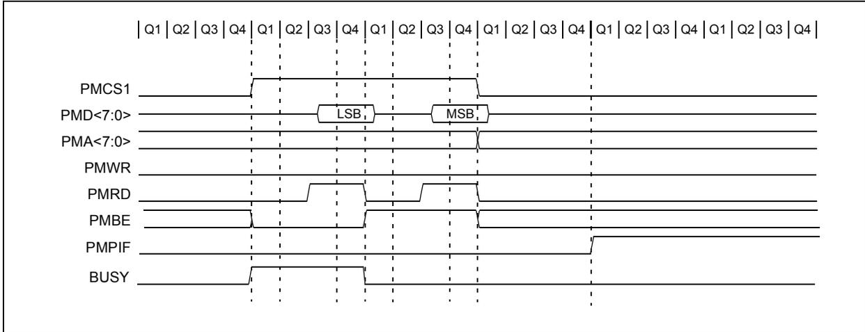
**FIGURE 11-22: WRITE TIMING, 16-BIT DATA, DEMULTIPLEXED ADDRESS**
