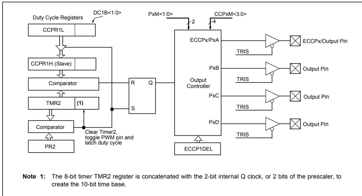
**Note 1:** The TRIS register value for each PWM output must be configured appropriately.
