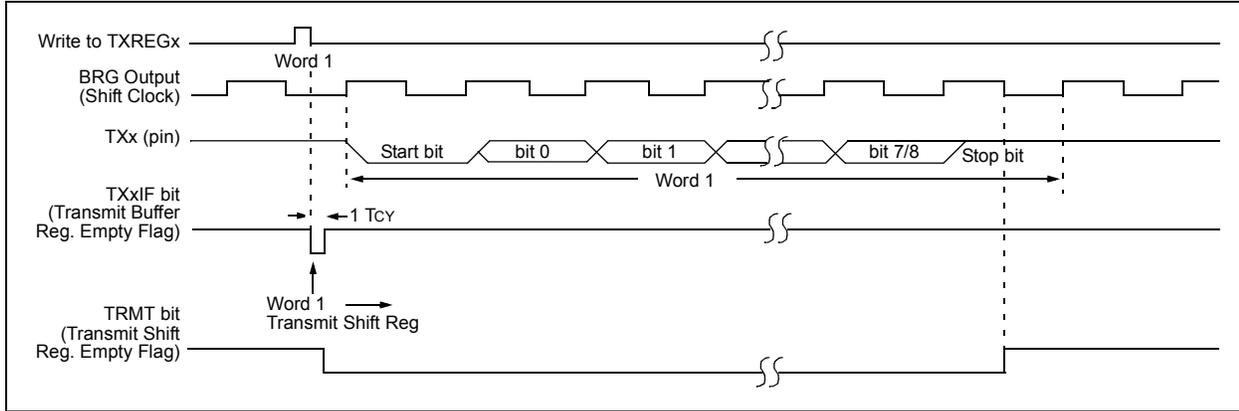
**FIGURE 21-5: ASYNCHRONOUS TRANSMISSION (BACK-TO-BACK)**
