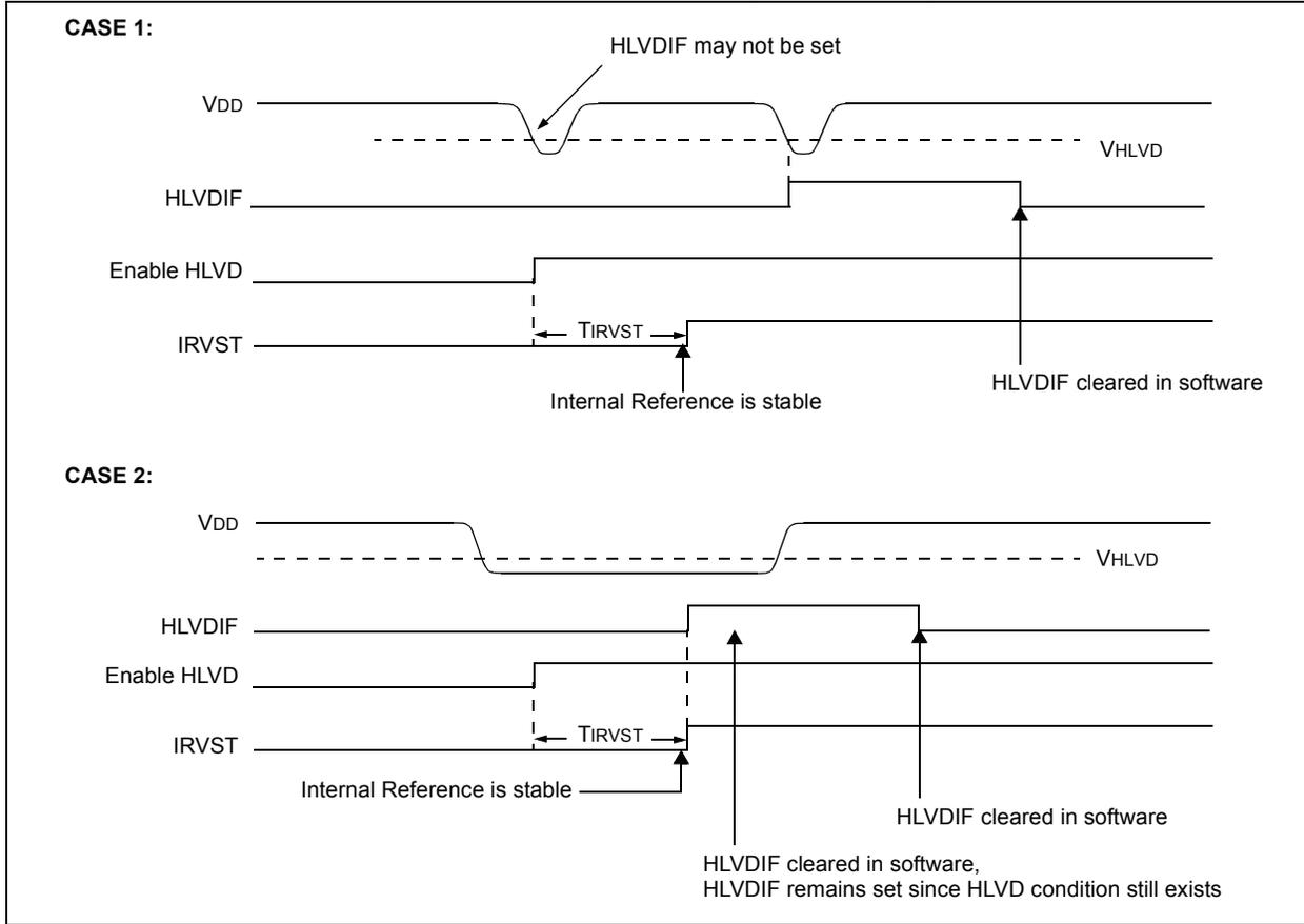
**FIGURE 26-3: HIGH-VOLTAGE DETECT OPERATION (VDIRMAG = 1)**
