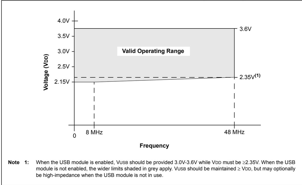
**FIGURE 31-2: PIC18LF47J53 FAMILY V<sub>DDCORE</sub> FREQUENCY GRAPH (INDUSTRIAL)<sup>(1)</sup>**
