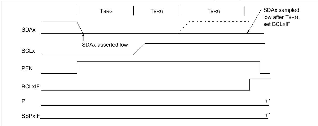
**FIGURE 20-34: BUS COLLISION DURING A STOP CONDITION (CASE 2)**
