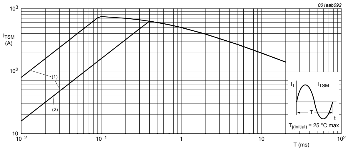
Fig. 4. Non-repetitive peak on-state current as a function of the number of sinusoidal current cycles; maximum values
